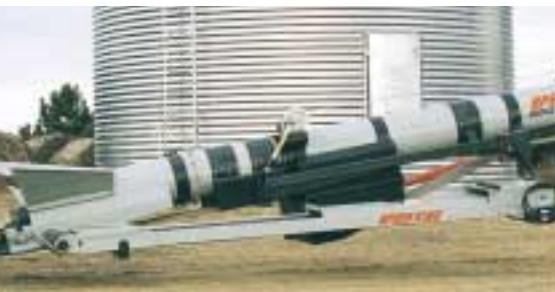
Slip-Pit™ in Transport Position
